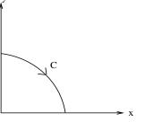
$$\begin{split} &\int_{C'} xy^2 dx - y^3 cy = \int_0^1 \left[ t(\sqrt{1-t^2})^2 (t)' - (\sqrt{1-t^2})^3 (\sqrt{1-t^2})' \right] dt \\ &= \int_0^1 \left[ t(1-t^2) - (\sqrt{1-t^2})^3 \frac{-t}{\sqrt{1-t^2}} \right] dt \\ &= \int_0^1 \left[ t(1-t^2) + t(1-t^2) \right] dt \\ &= 2\left( \frac{t^2}{2} - \frac{t^4}{4} \right) \bigg|_0^1 = 2\left( \frac{1}{2} - \frac{1}{4} \right) = \frac{1}{2}. \end{split}$$
